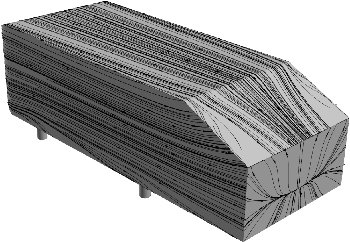
Figure 199 The Arrows & Lines display type for Surface Flows provides insight on the direction of the flow near the wall. Shown here is the rear of a notional car (the Ahmed body).
