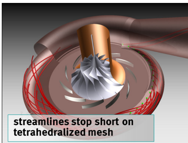
Figure 8 Streamline improvements resulting from Arb Poly Interpolation
