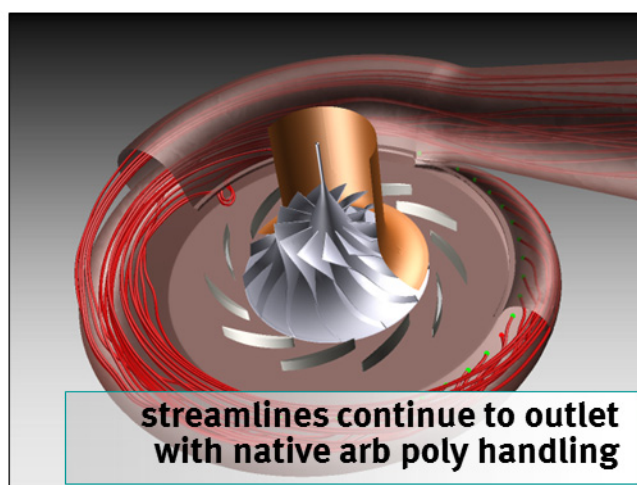
Figure 8 Streamline improvements resulting from Arb Poly Interpolation
